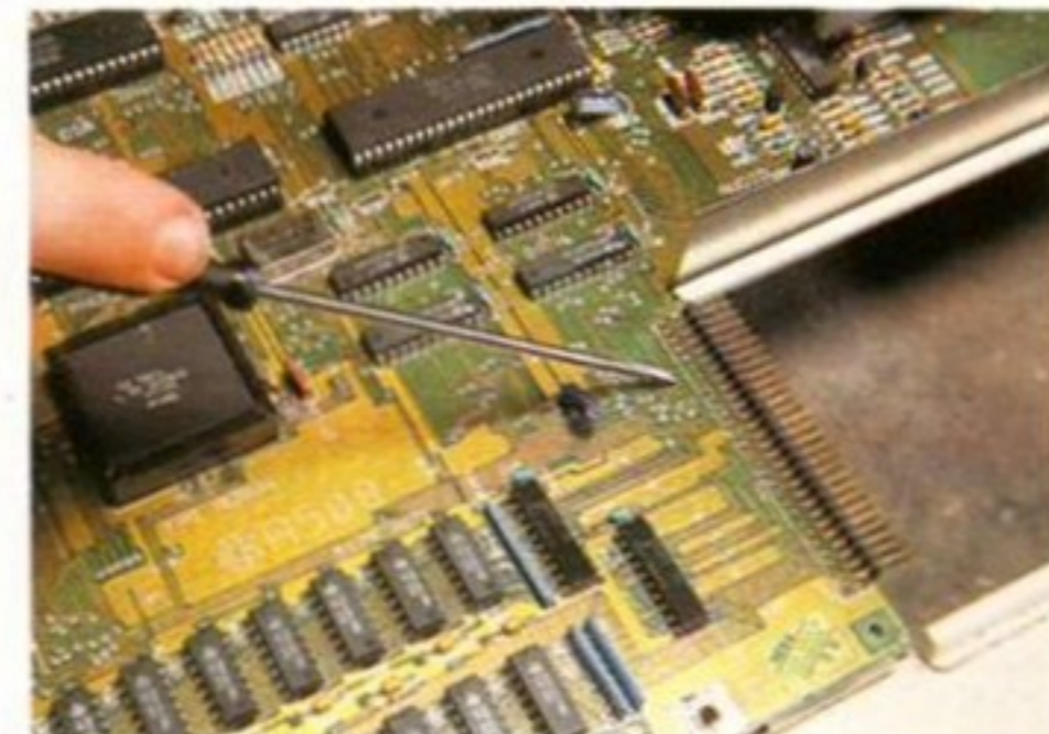
Revision 5 machines need the indicated track cut - on revision 6A machines this is clearly marked as JP7A
